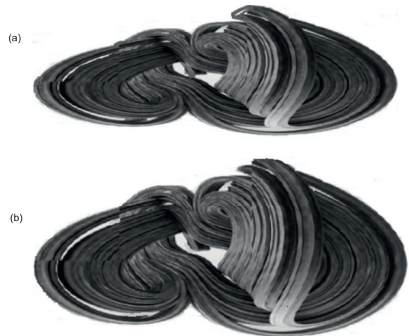
Fig. 3. Rough representation of a four-scroll attractor of system (1.3) in a chaotic state, with the control parameters a = 4, b = 1, c = 5, d = 5, e = 10, f = 1 and \alpha = 1.0 .
