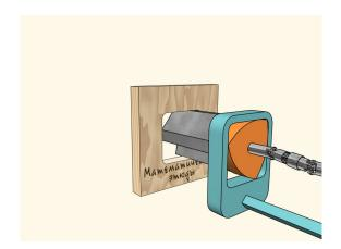
The cross-section of the orange piece is a Reuleaux triangle, which allows one to drill a square hole.
